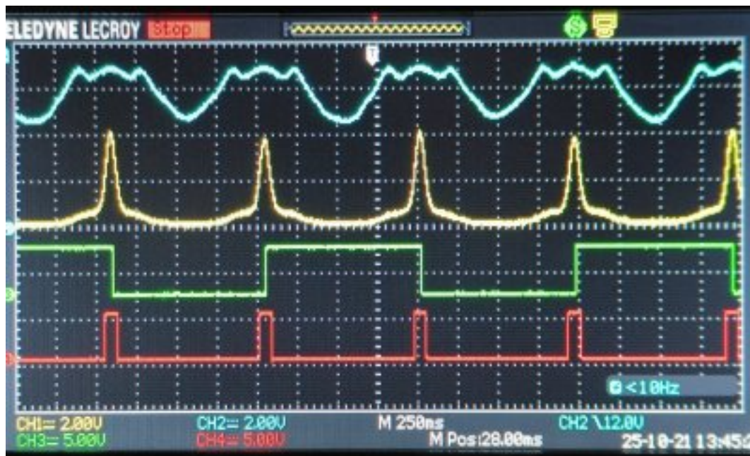
Fig 2. The signals from the Capacitive detection.
